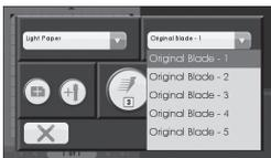
If you have any previously defined tools set up for your Cricut Expression 2 machine, you can use this dropdown menu to select this tool and proceed by loading your mat and pressing the **Cut** button. You can also select one of the pre-defined tools in the dropdown menu. The number after the name of each of the pre-defined tools specifies the depth that should be set for that tool on the blade assembly prior to cutting.
